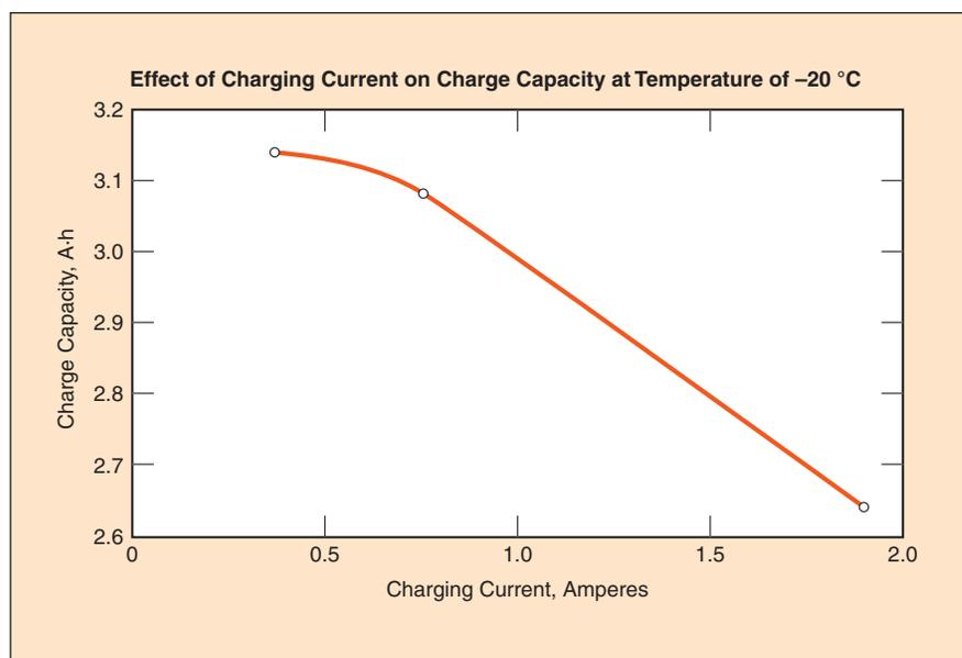
The **Charge Capacity** attainable by charging a representative Li-ion battery at constant current decreases with increasing current if the end-of-charge battery-terminal voltage is limited to a nominal full-charge value, because of internal ohmic voltage drop.
