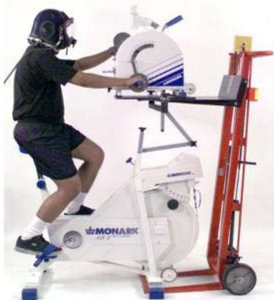
Dual-Cycle Ergometer used for Exercise-Enhanced Prebreathe
