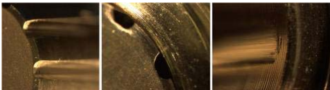
Figure 17: Passed pressing trial results with 40 \mu\text{m} oversize
