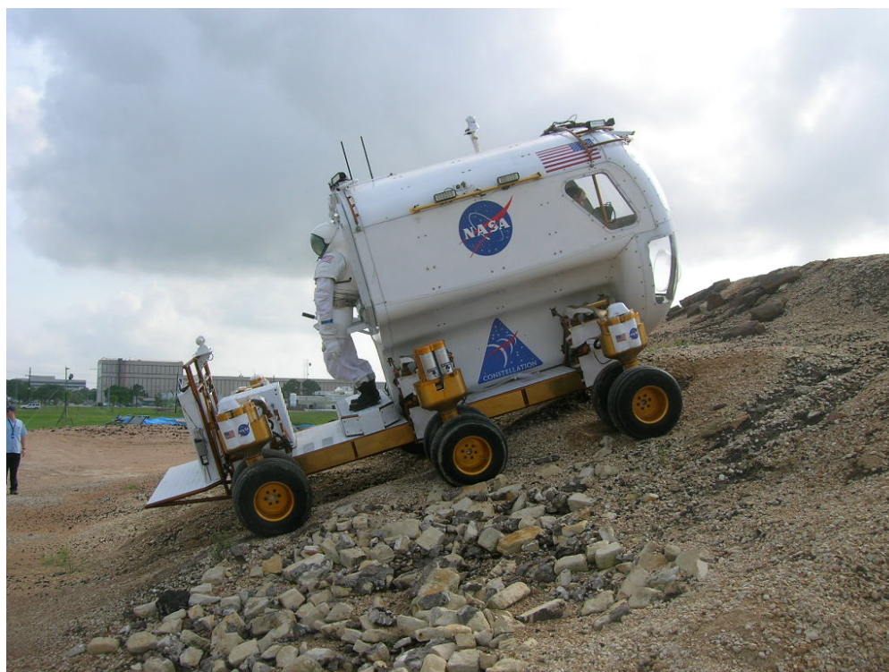
Figure 14. LER with New Gearbox Climbing a Steep Grade
