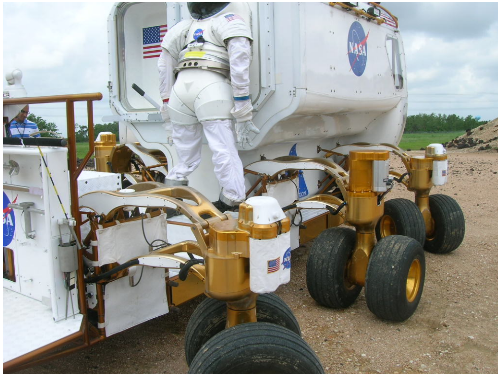
Figure 12. Chariot in LER Form, Starboard Center Wheel Pod with New Gearbox
