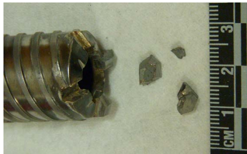
Figure 11. Failed Bit after High Energy Basalt Testing
