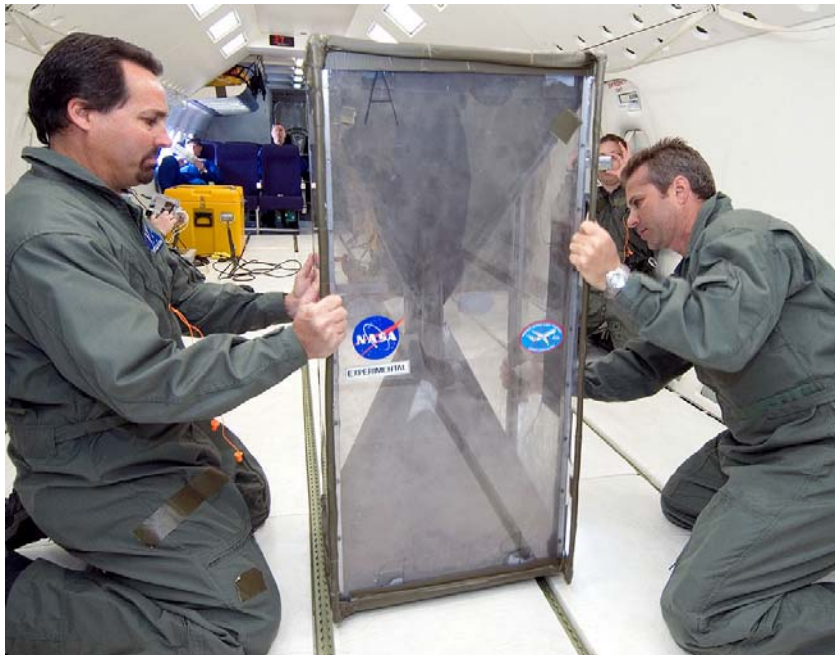
Figure 5: Flight experiment in May 2008 to test the flow of regolith simulant inside a hopper under reduced gravity conditions.
