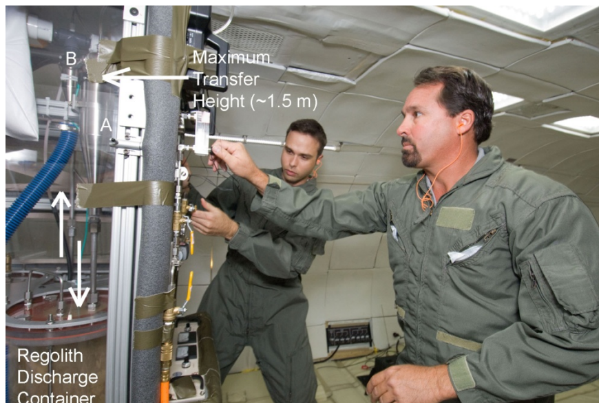
Figure 11: Photo of the RGF experiment showing Tephra that fell from cyclone A into the Regolith Discharge Container. The Tephra flowed vertically upward along a convey pipe from the eductor located at the bottom of the Supply Container (not visible in photo). The convey pipe had a vertical-to-horizontal transition which connected it to the inlet of cyclone A in Fig. 9. The gas exhaust from cyclone A became the input for the smaller cyclone B, which discharged dust into the blue hose shown in the picture. The exhaust from cyclone B passed through HEPA filter bags before exiting into the transparent containment box, which had a secondary HEPA filter that allowed the filtered air to enter into the aircraft cabin.
