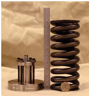
Figure 3. Piston/Cylinder Actuator (Left), And Spring It Compressed (Right) During Actuation
