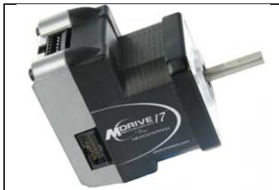
Figure 12. MDrive 17 Motor and controller (300 grams)
