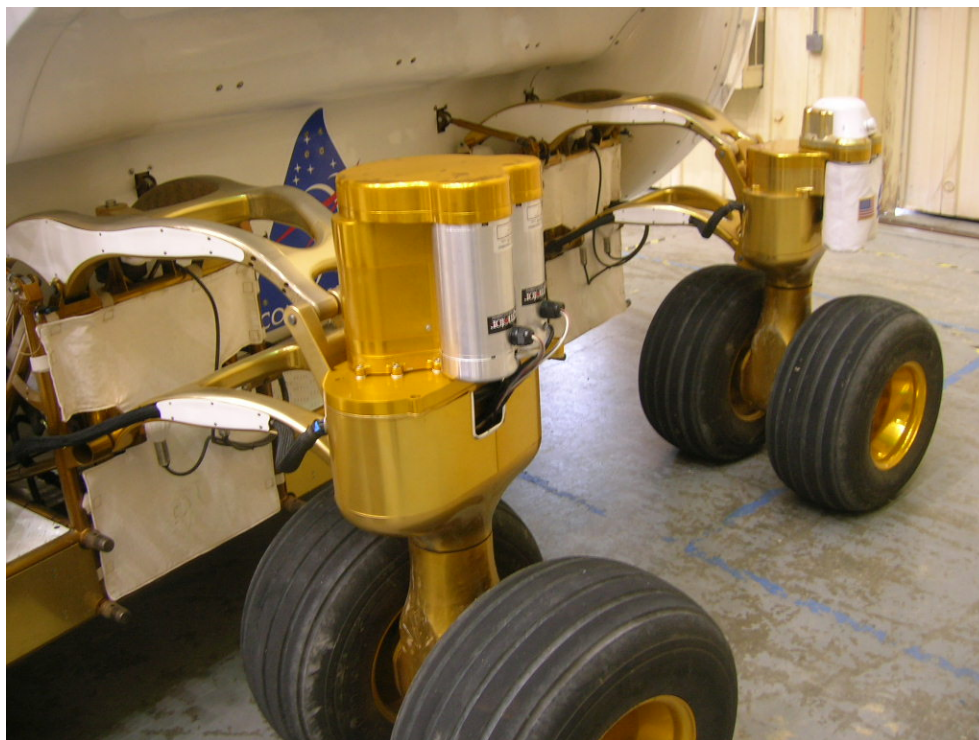
Figure 13. LER Starboard Center Wheel Pod, New Gearbox Close-up
