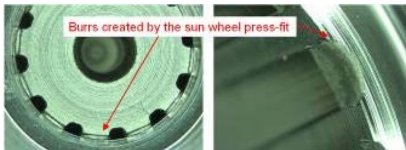
Figure 16: Failed pressing trial results
