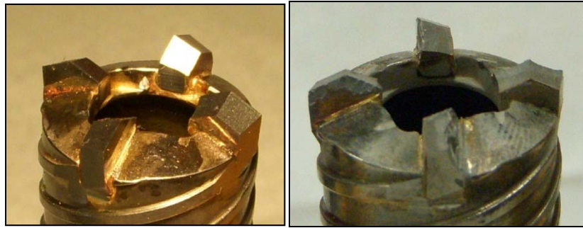
Figure 10. New Bit and Chipped Bit after Basalt Testing
