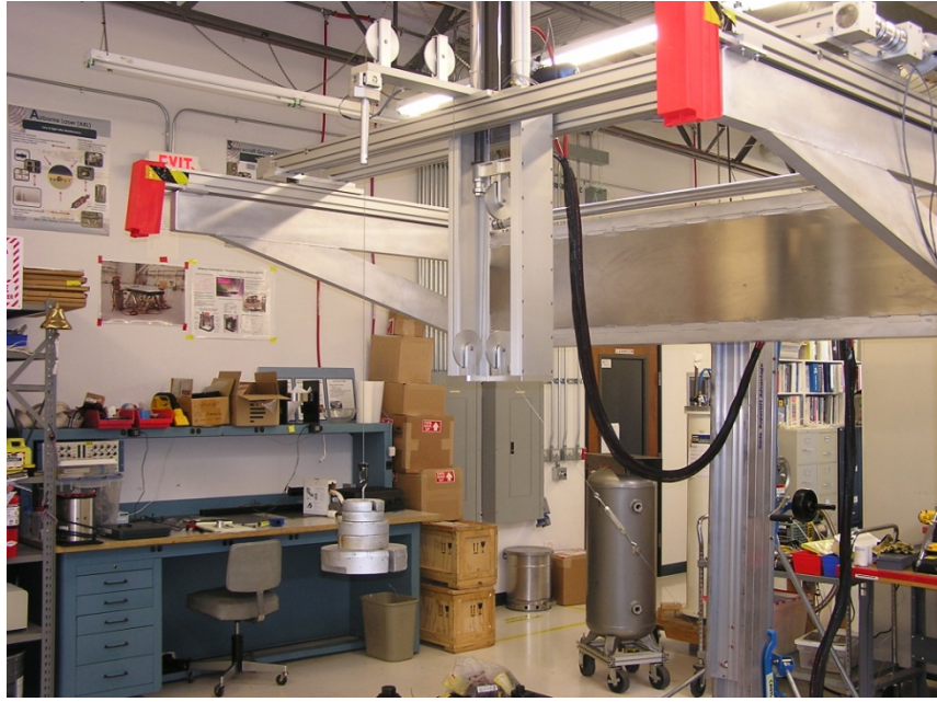
Figure 8: WAGM supporting 360.26-N (80.99-lb) payload
