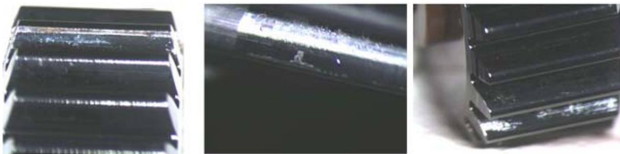
Figure 19: Coating damage after vibration
