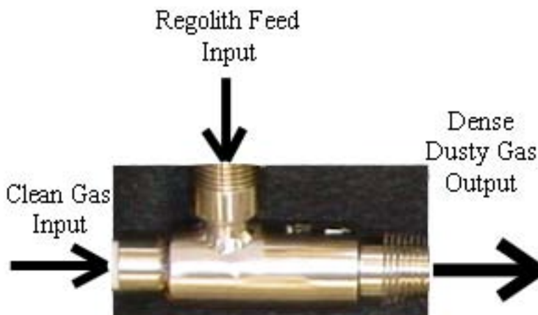
Figure 10: An eductor produces a dense flow of dusty gas by creating a partial vacuum via the Venturi effect that entrains lunar regolith feedstock material into a flow of clean dry air.
