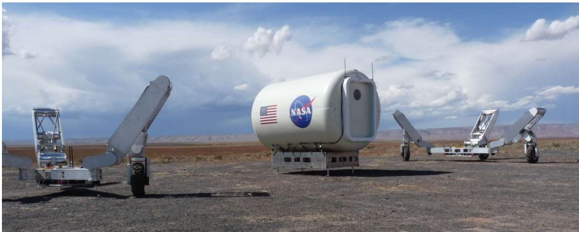
Figure 2. Two Tri-ATHLETE vehicles prior to docking to the mobile habitat / pallet
