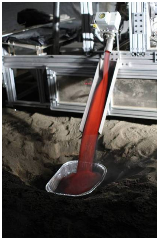
Figure 4: Hot Tephra (~1000 C) flowing out of Gemco, Inc valve attached to the bottom of the ROxygen I Reactor.
