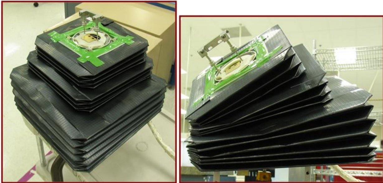
Figure 8. Multilayer Insulation (MLI) Blanket
