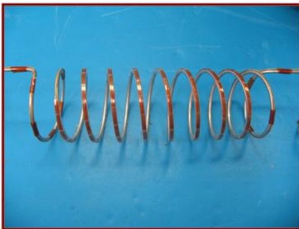
Figure 4. Outer Propellant Tubing with Heater
