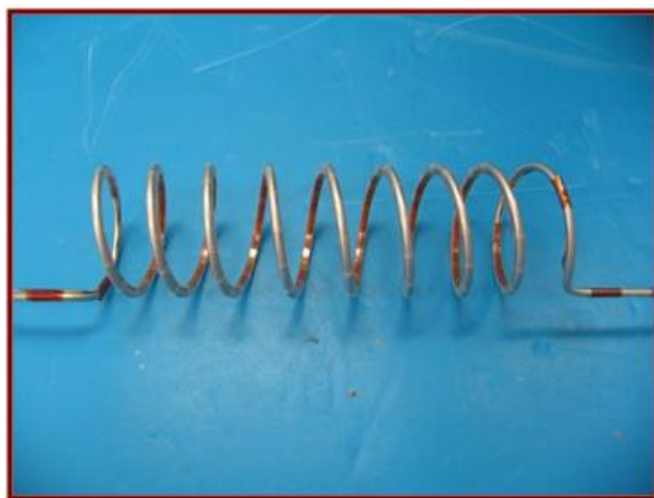
Figure 5. Inner Propellant Tubing with Heater
