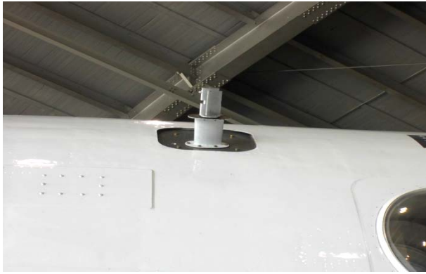
Figure 7. Close-up View of TAMDAR Installed.
