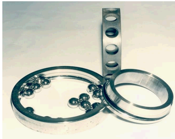
LOW THRUST LOADED BEARING FROM BSMT. CAGE NOT DAMAGED, MINOR SURFACE DEGRADATION ON RINGS, BALLS SLIGHTLY WORN
