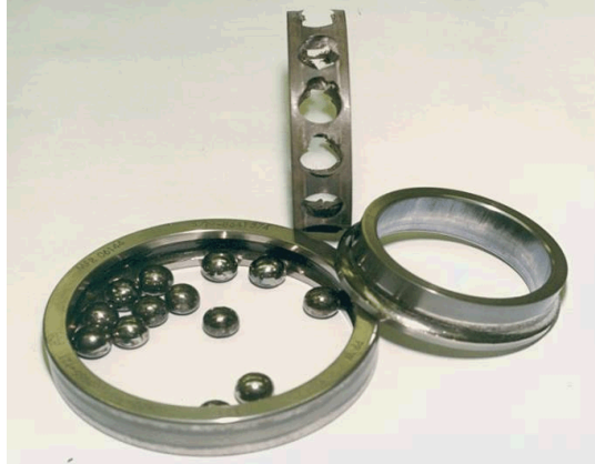
HEAVILY WORN BEARING FROM THERMAL MARGIN TEST. THIS BEARING HAS HIGH THRUST LOADING DURING RUNS. MAJOR SURFACE DISTRESS ON RACES, CAGE DAMAGED, AND SEVERELY WORN STEEL BALLS
