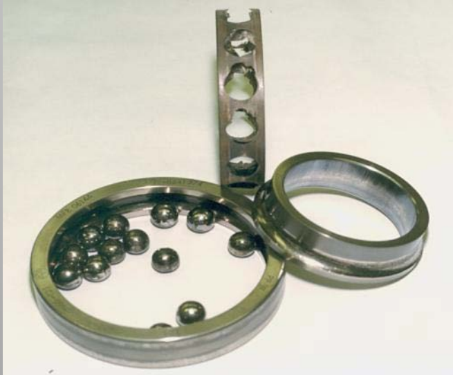
Heavily worn born bearing from margin test, high thrust load
