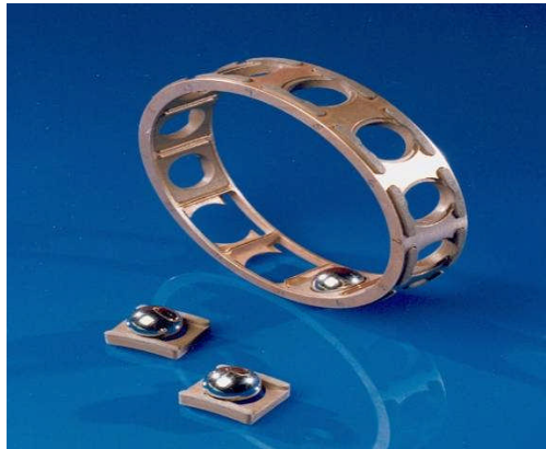
BEARING CAGE WITH BRONZE POWDER/PTFE INSERTS AND BRONZE HOUSING TESTED IN BSMT
