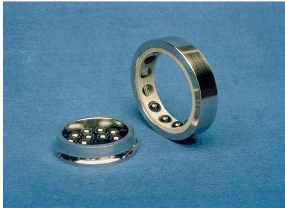
SSME HPOTP BEARING WITH SILICON NITRIDE BALLS AS RUN IN THE BSMT
