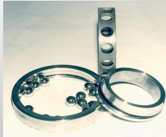
Bearing from margin test, low thrust load
