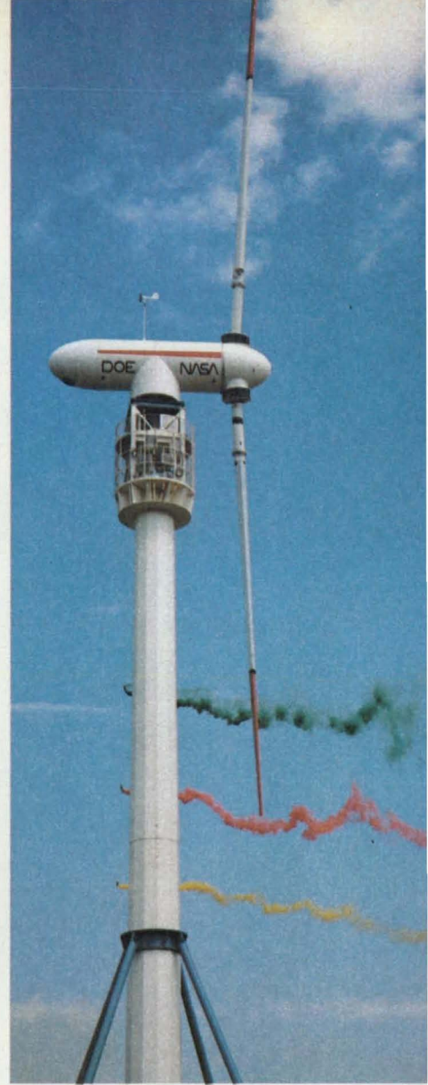
The Mod-O wind turbine generator is located at Lewis' Plum Brook Station. Smoke tests reveal the true pattern of wind as it flows through the turbine blades.
