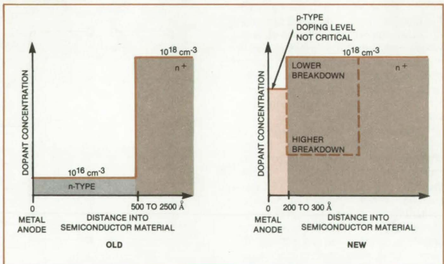
Doping Profiles of old and new devices are compared. A high-breakdown-voltage option is provided in the new structure.
