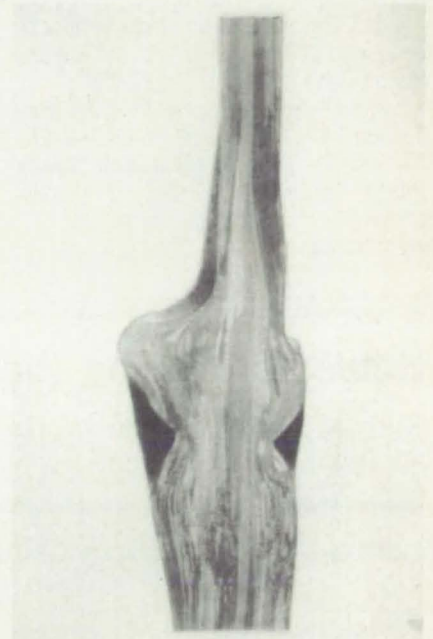
GRAIN STRUCTURE OF ODS TURBINE BLADE
