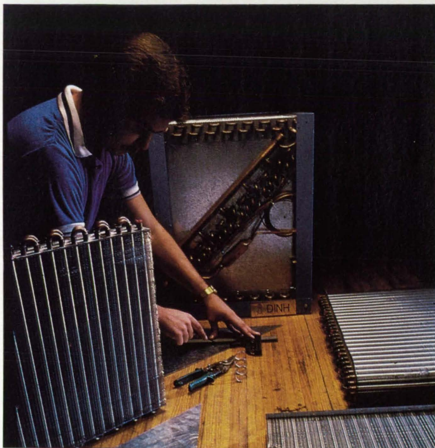
The Dinh Company, Alachua, FL, developed a heat pipe dehumidification system that can double the moisture removal capacity of any air conditioner. NASA's Southern Technology Applications Center assisted with the research necessary to develop the system, whose components are shown here.
