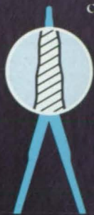
Missile fin cross-section showing "terraced" profile
