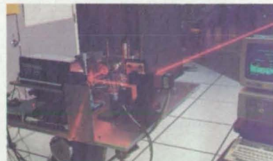
Currently under evaluation at NASA's Johnson Space Flight Center, this laser-based tracking system may help dock spacecraft with the Space Station a few years from now. Note the three mirrors on the target to the right. The tracking system is described on page 12.
