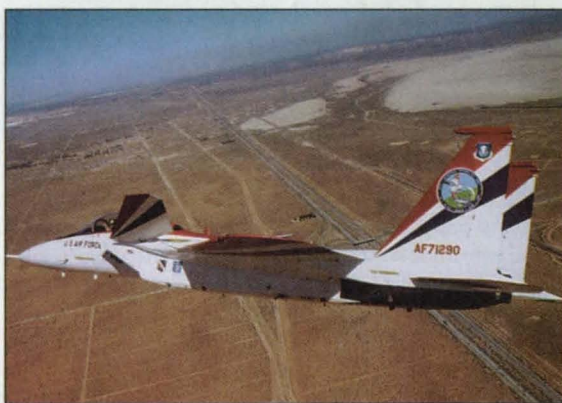
The Advanced Control Technology for Integrated Vehicles (ACTIVE) program at Dryden uses specially modified F-15s to test how advanced thrust vectoring engine nozzle technology can improve the aircraft's performance during cruising flight or in maneuvering.
