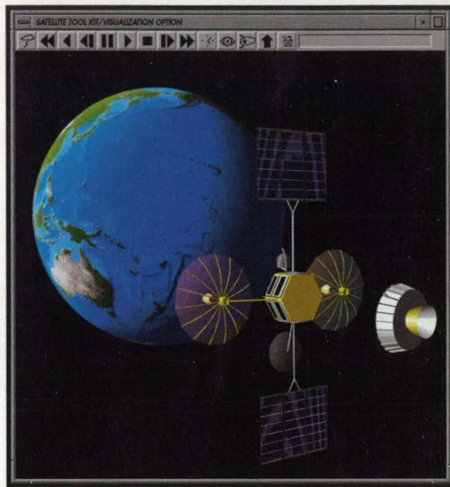
A Tracking and Data Relay Satellite (TDRS) just after Inertial Upper Stage (IUS) separation.
