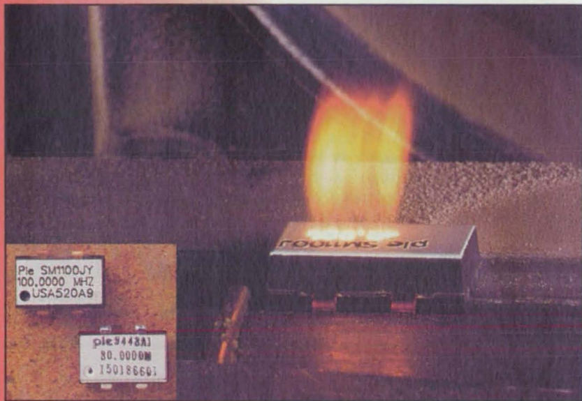
Inset: Comparison of print quality on ink-marked (lower) and laser-marked (upper) chips
