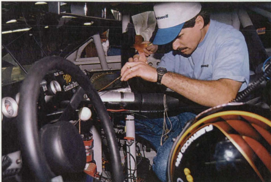
A Rockwell International engineer installs a thermocouple device inside the Penske Ford to measure how well the space shuttle thermal blanket material would work to reduce heat in the driver's cockpit under race track conditions.
