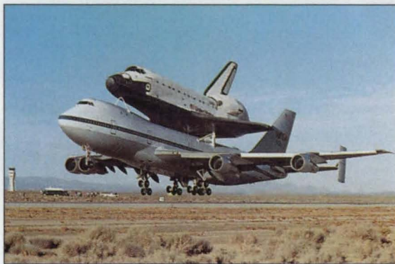
Modified Boeing 747s are used as Space Shuttle Carrier Aircraft (SCA) to take the shuttle orbiters back to the launch site at Kennedy Space Center in Florida after landing or servicing at another site. The NASA 905, the first SCA in service, is shown leaving Dryden with the orbiter Atlantis.
