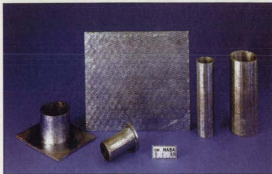
Research at NASA Lewis has produced a low-cost approach to fabrication and joining of composites with 3D architectures, such as silicon carbide-based fiber-reinforced composites.
