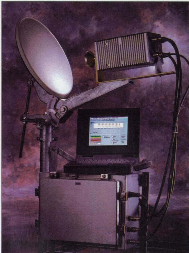
The smallest of the ACTS communication satellites, the Ultra Small Aperture Terminal (USAT) features a space-saving 14-inch antenna. USAT is used for interactive distance learning and remote medical tele-imaging.
