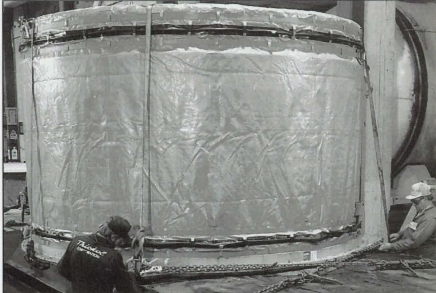
A Flexible Cover prevents rusting of a large steel cylinder (part of the case of a solid-fuel rocket motor) by enclosing it in dry air.
