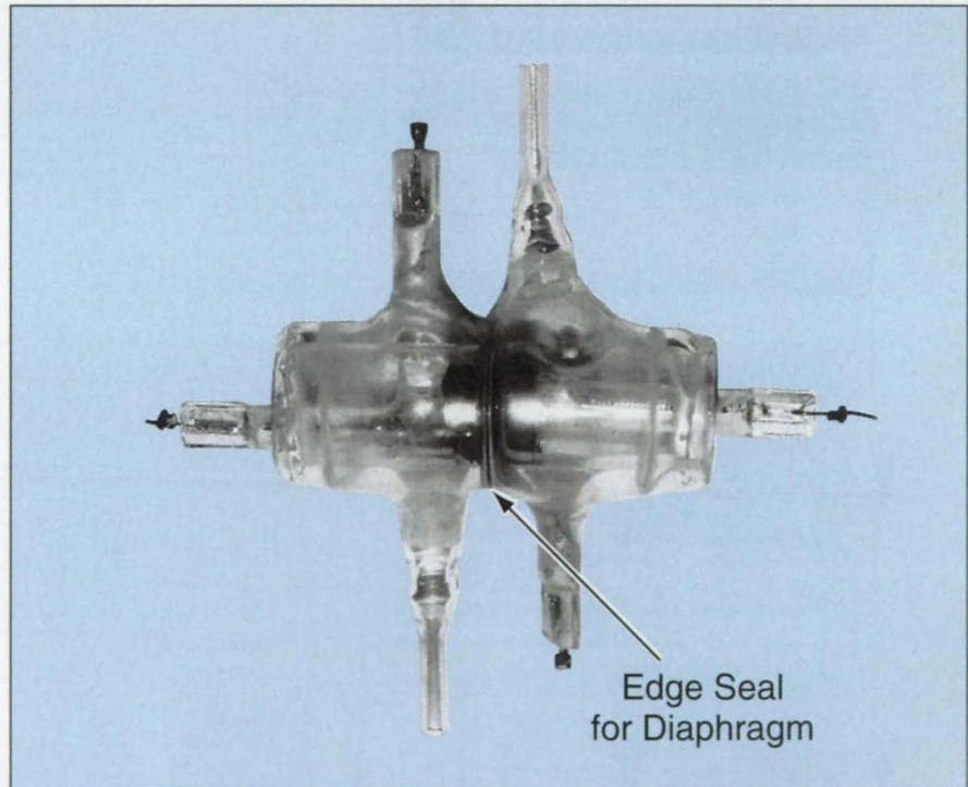
This Prototype Gauge includes a quartz housing and hermetically sealed electrical feedthroughs similar to those of halogen lamps.
