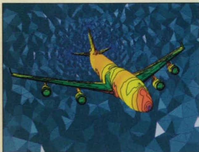
TetrUSS aerodynamics analysis and design software, developed at NASA Langley, enables fluid mechanics analysis for low-speed through supersonic aircraft such as the B747 shown here.
