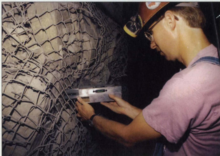
Figure 1. Metal strips along one side or the bottom of the Geolaser can be extended to allow the instrument to be placed in a tight opening.
