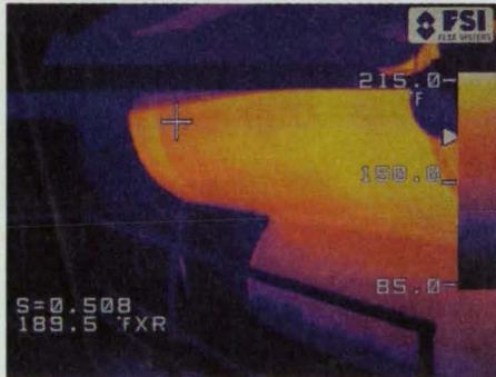
Despite a hot, humid environment, the IQ 812 system confirms uniform moisture content in this high-speed paper production process.
