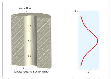
The **Superconducting Electromagnet** generates a static magnetic field with a vertical gradient. For water or other substances of diamagnetism, the gradient magnetic field opposes or aids the gravitational body force by an amount that varies with position along the bore.
