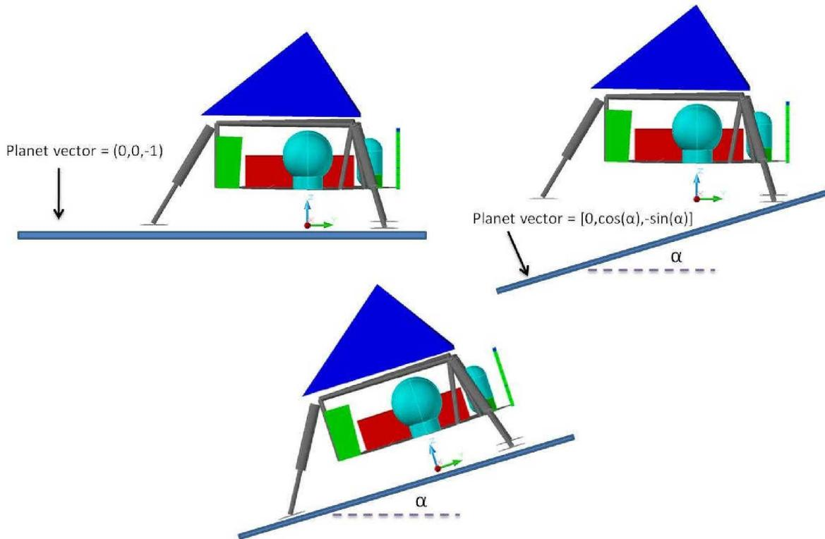
Figure 6: Surface Modeling using Thermal Desktop Orbit Command.
