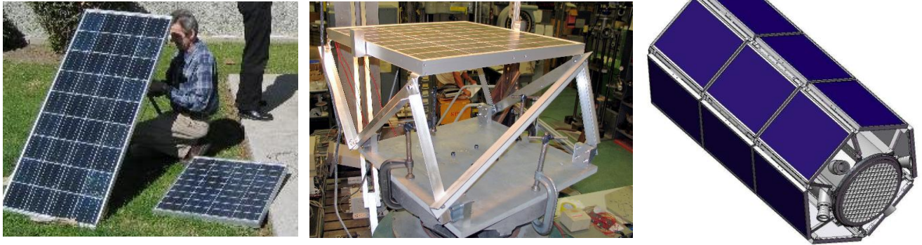
Figure 6: Solar Panels, Mounting Structure, and Configuration on COTSAT-1
