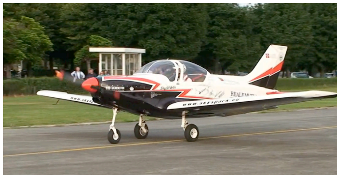
DigiSky SkySpark – 2009 Li-Polymer battery 155 mph, 8 minute flight
