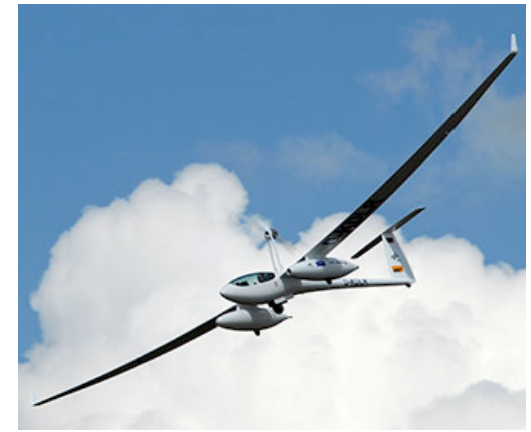
Antares DLR-H2 – 2008 PEM fuel cell + battery 106 mph, 10 min flight, 465 mi range
