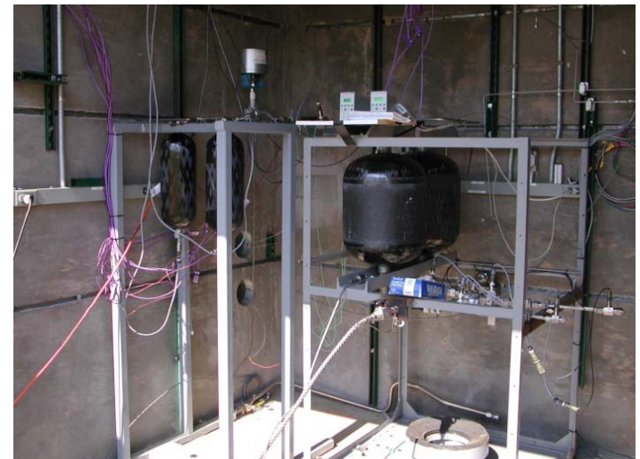
High pressure regulator test setup at MSFC
