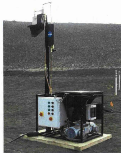
Figure 1. The Pneumatic Regolith Feed System demonstrated for the 2010 ISRU Carbothermal field test on Mauna Kea.
