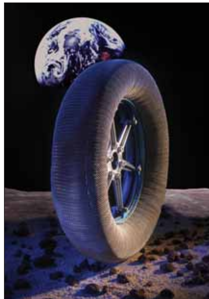
The Spring Tire , co-invented by NASA Glenn Research Center and the Goodyear Tire & Rubber Company. This airless, rubberless tire is capable of contouring to the rocky surface of the Moon, yet consumes far less energy than an Earth tire. Photo Credit — Aaron Vandersomers/Goodyear
