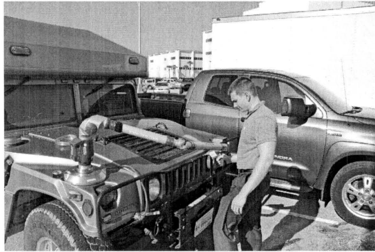
Figure 11 Using the FAROarm to Collect Hummer Data
