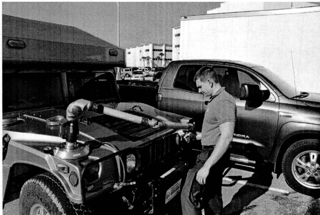
Figure 13 - Using the FAROarm to Collect Hummer Data
