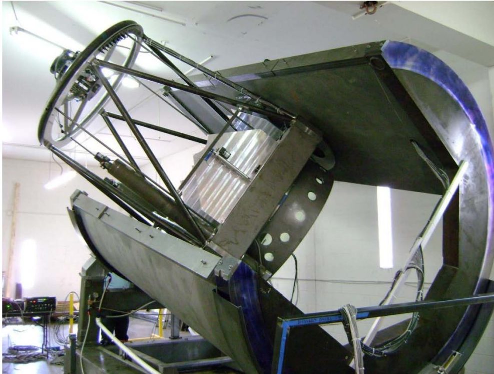
Figure 4. – Double horseshoe mount of the type to be used on the MCAT provides a stable equatorial mount for a low latitude site with the added benefit of unobstructed north polar and south horizon access.
