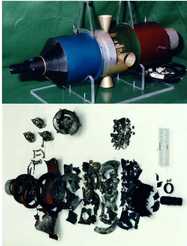
Figure 6. – Simulated Satellite impacted by 1-cm steel ball along the axis of the satellite at 7 km/sec velocity.
