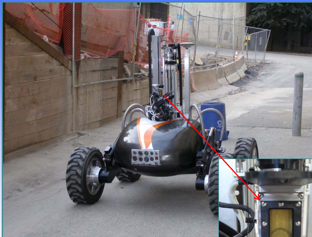
Spiral EDS mounted on RESOLVE rover
