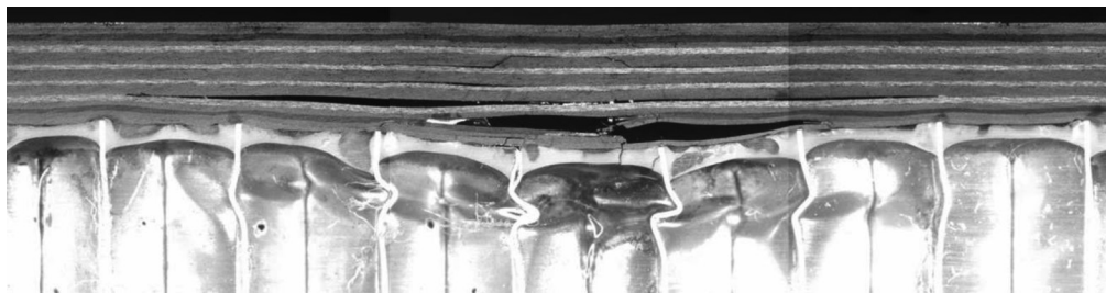
Figure 19. 6 ft-lb, 0.5-in-diameter impactor.
