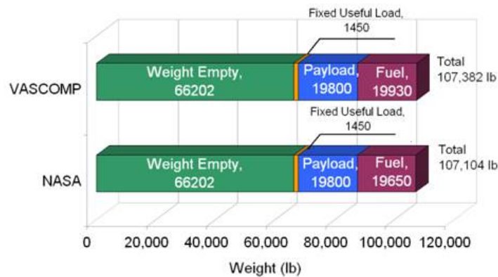
Figure 7-34. LCTR2 weight composition (excluding fuel weight).
