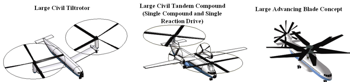
Figure 7-31. NASA's heavy-lift rotorcraft configurations
