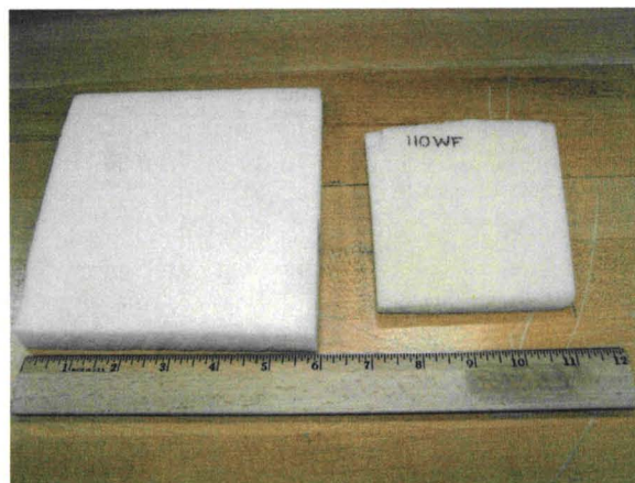
Figure 2: Two samples of 110 WF Rohacell Foam were vacuum dried and subjected to moisture uptake testing in an environmental chamber.
