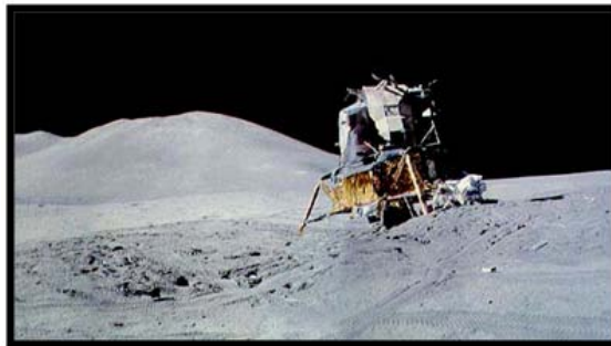
Fig. 1: Apollo 15 Lunar Module Falcon at the Hadley-Apennine landing site with read pad in a crater
