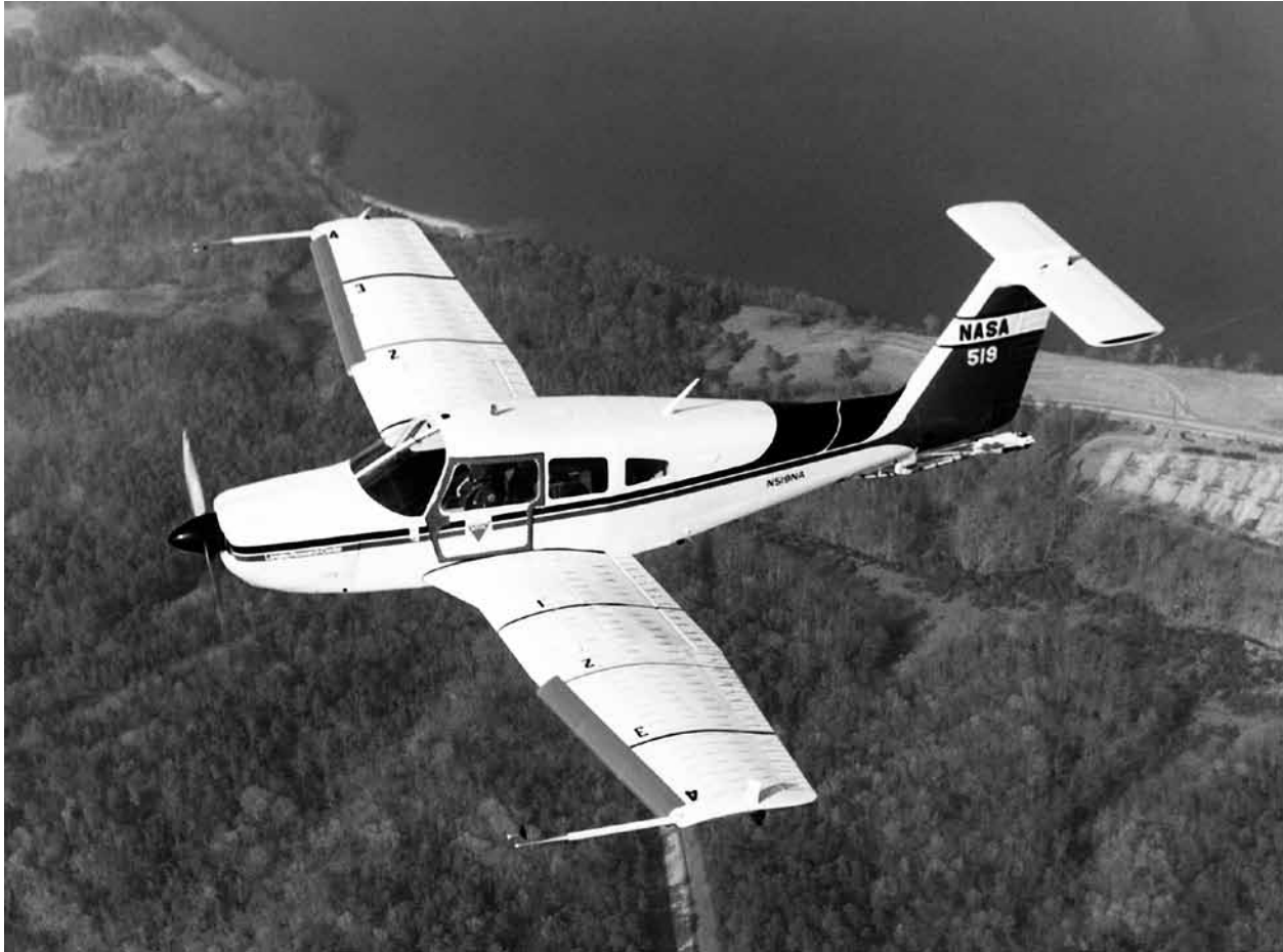
This T-tail low wing NASA research aircraft displays the discontinuous wing leading-edge modification that significantly increased the spin resistance of configurations in NASA's stall/spin program. Radio-controlled model results for another low wing configuration agreed well with full-scale flight results.
