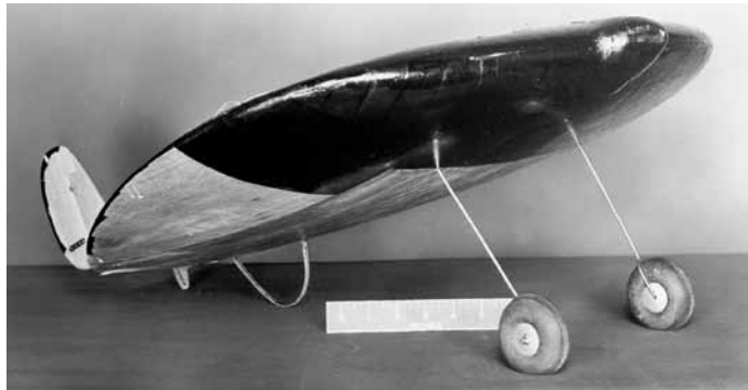
Original unpowered free-flight model configuration of the V-173 “Flying Pancake” as it entered testing in the Langley 12-Foot Free-Flight Tunnel in 1939. Initial test results were very unsatisfactory and required extensive redesign of the tails and control surfaces.
