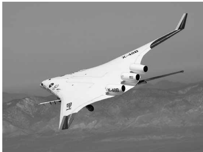
The Boeing X-48B Blended Wing-Body configuration in flight at NASA Dryden. The configuration has undergone almost 15 years of research, including free-flight testing at Langley and Dryden. The stinger visible at the rear of the model is used for deployment of a parachute for emergency spin and tumble recovery.
