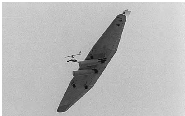
Stanford University supported the NASA Ames Research Center with radio-controlled, free-flight model testing of several oblique wing models. Here, a 20-foot-span oblique flying wing model powered by two ducted fans is undergoing flight evaluations.
