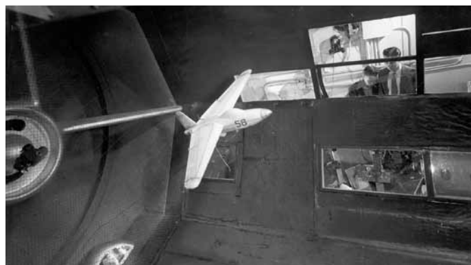
Free-flight test of a swept-forward wing, tailless fighter design known as the Air Material Command MCD-387-A in the Langley 12-Foot Free-Flight Tunnel. The evaluation pilot is visible in the enclosure at the lower left, while the two tunnel operators controlling airspeed and tunnel tilt angle are at the right.
