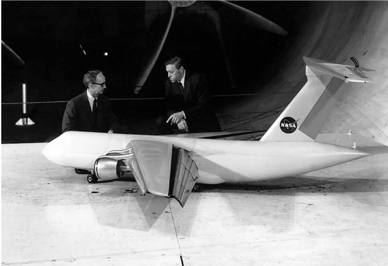
John P. Campbell, left, inventor of the externally blown flap (EBF) concept, and Gerald G. Kayten, of NASA Headquarters, pose with a generic free-flight model of an STOL configuration at the Full-Scale Tunnel. Large slotted trailing-edge flaps were used to deflect the exhaust flows of turbofan engines to induce extremely high lift at low speeds. Note the nose-down tilt of the engine nacelles and the high T-tail used to avoid the large downwash variations behind the wing in STOL conditions.
