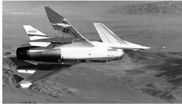
The HiMAT remotely piloted research vehicle flies over Edwards Air Force Base. In its role as an advanced technology demonstrator, the vehicle incorporated a highly sophisticated flight control system, a canard, winglets, aeroelastic tailoring, and relaxed static stability.
