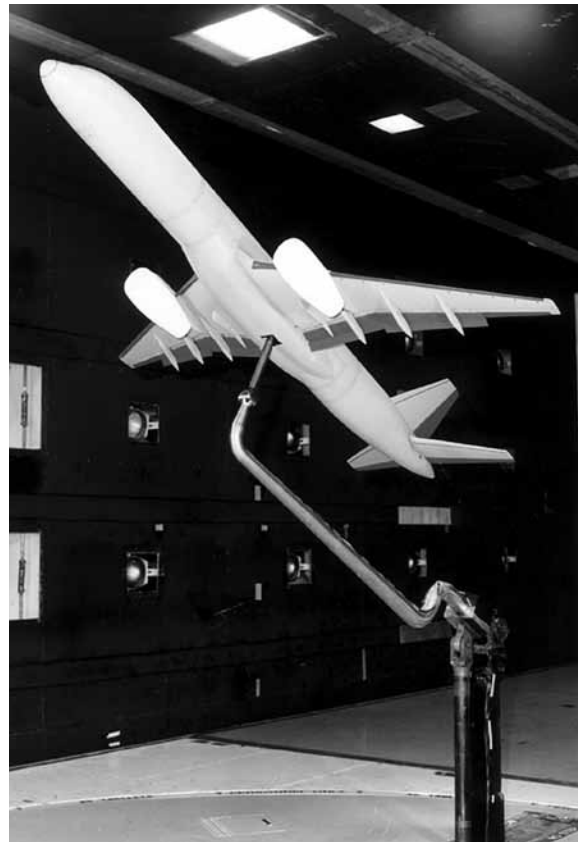
In preparation for model flight tests in the AirSTAR project, Langley has conducted conventional and dynamic force tests in the 14- by 22-Foot Tunnel to measure the aerodynamic characteristics of the configuration.
