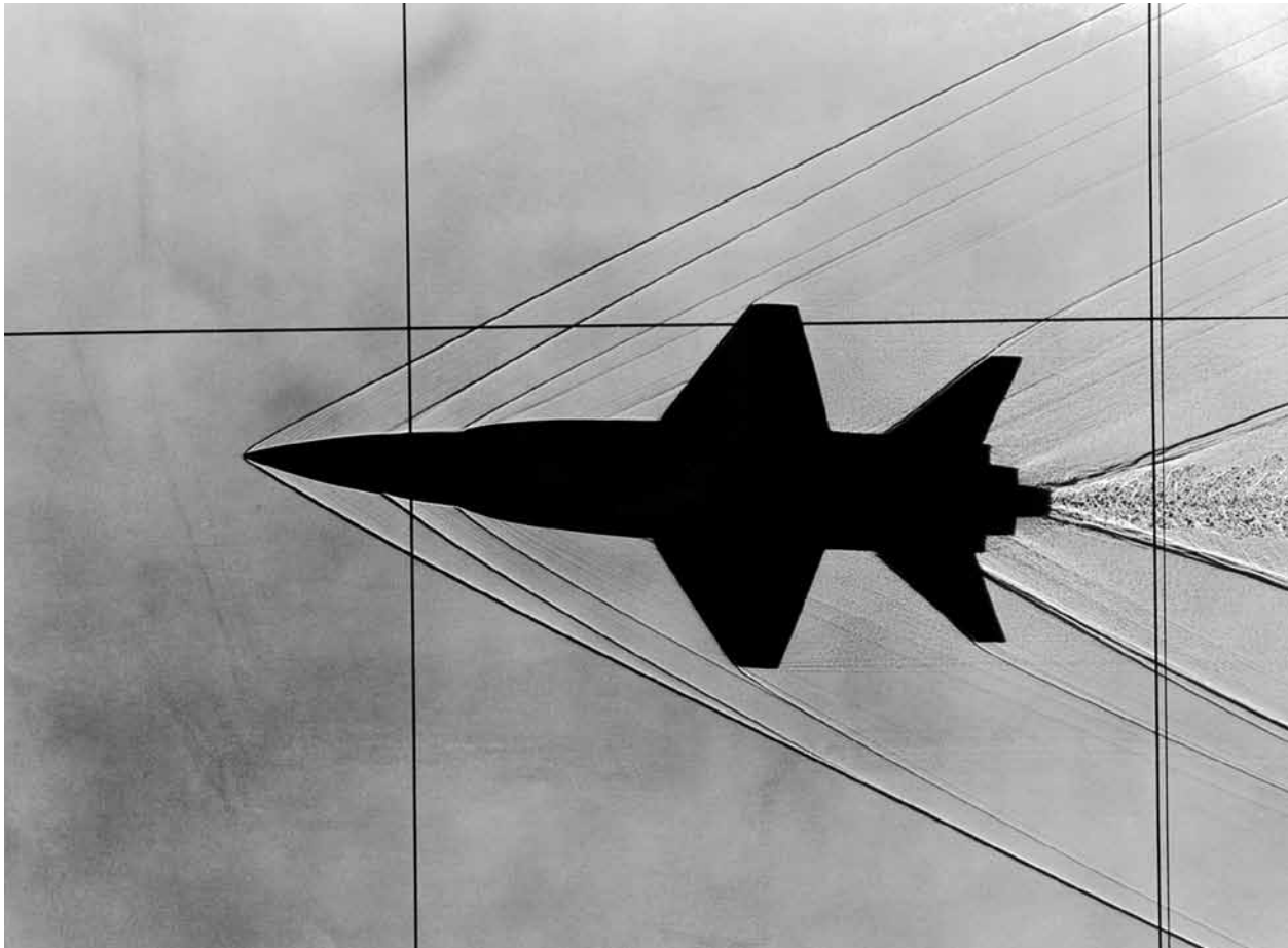
Supersonic free-flight test of a model of the X-15 research airplane in the Ames Supersonic Free-Flight Facility. The locations of shock waves emanating from the fuselage, wing, and tail of the model are crisply defined by the shadowgraph technique.
