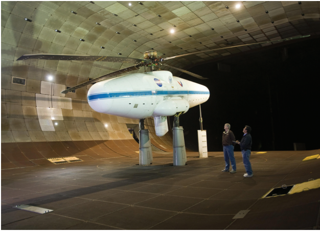
Figure 69. UH-60A Airloads rotor in the 40- by 80-Foot Wind Tunnel.
