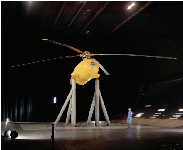
Figure 63. H-34 airloads rotor in the 40- by 80-Foot Wind Tunnel.
