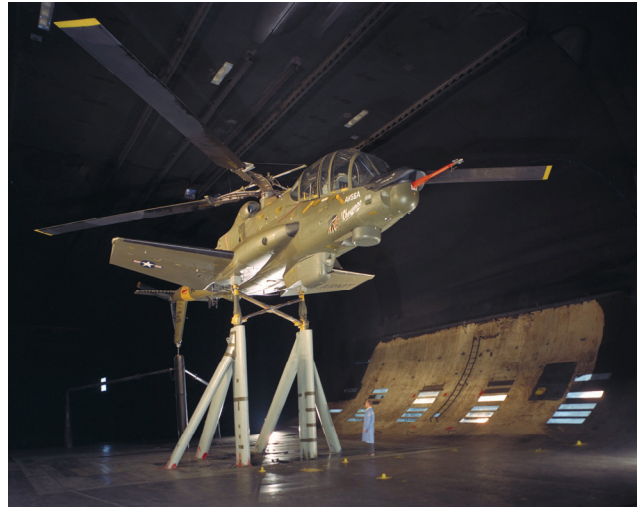
AH-56A in wind tunnel
