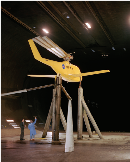
XH-51A stopped rotor test
