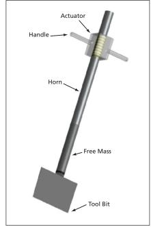
The **Ultrasonic/Sonic Jackhammer** is driven electrically instead of pneumatically. It offers several advantages over a conventional pneumatic jackhammer.
