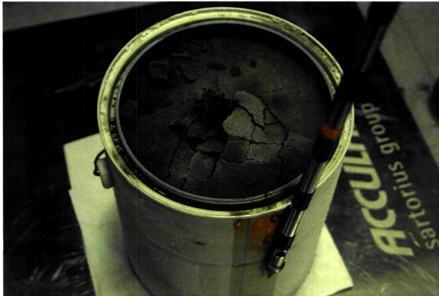
Figure 9. Fractured surface of can #4. Shaft demonstrates depth of penetration.
