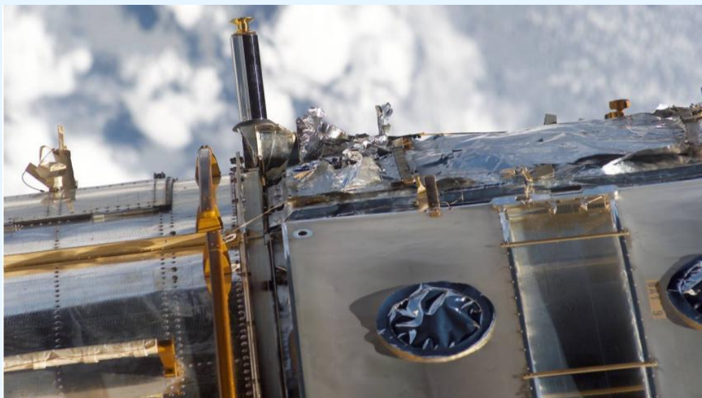
On-orbit insulation degradation and embrittlement
