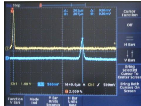
Image 4. Measuring Time off the Oscilloscope. The vertical cursors are placed at the peak of each wave. These peaks indicate when the particle passed by each sensor. In this picture the time it took for the particle to move from one sensor to the next was 262 microseconds.
