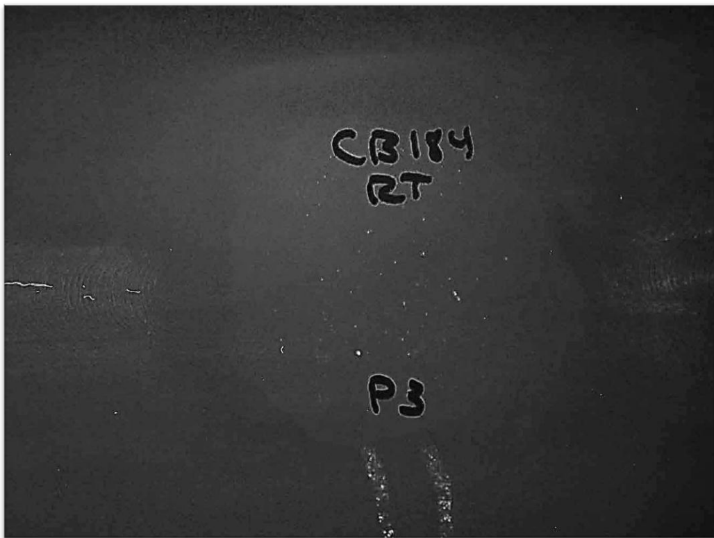
Figure C4 Round indications located lower left quadrant of the plug.
