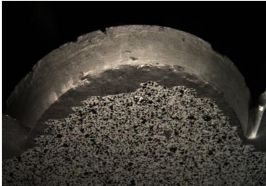
Figure 3.39 Fracture surface around plug with little or no bond to weld.
