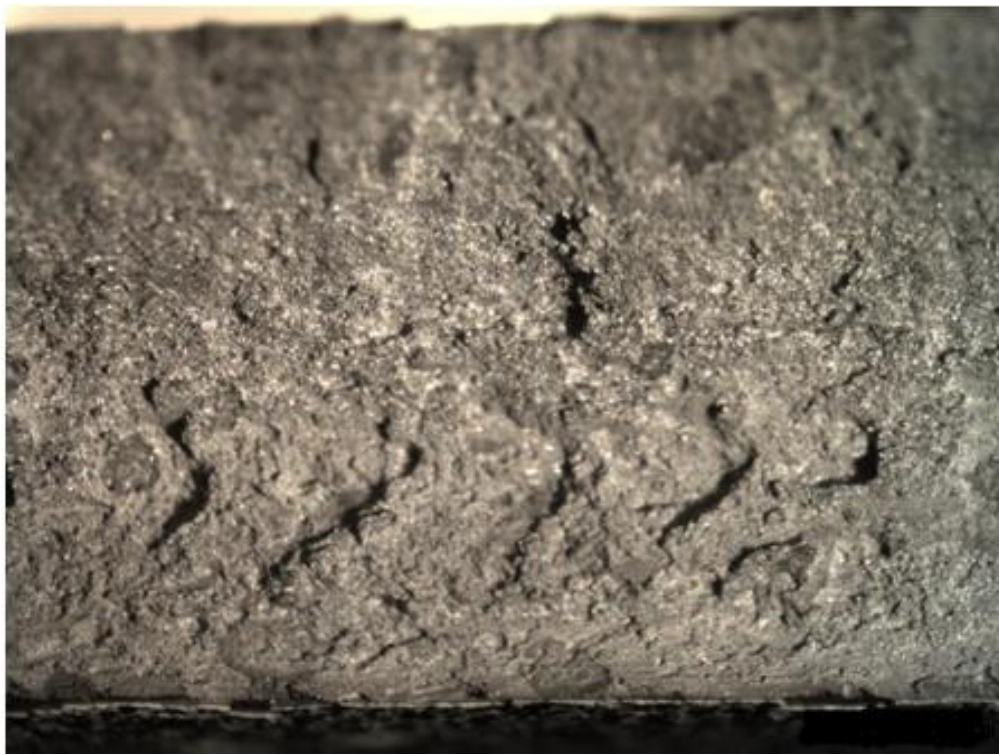
Figure 3.41 Ductile fracture surface of SR-FSW.
