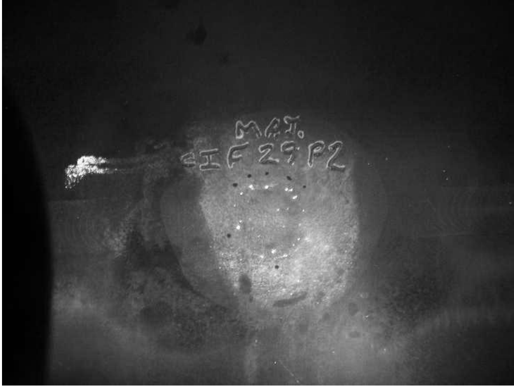
Figure C5 Round indications marked with red marks.
