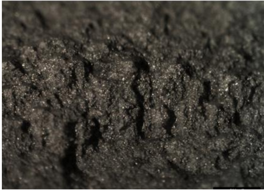
Figure 3.38 Rough ductile surface on the surface of the plug fracture area of the sample that failed through the plug.
