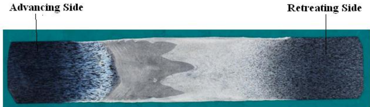
Figure 3.1 Macrograph of initial weld.
