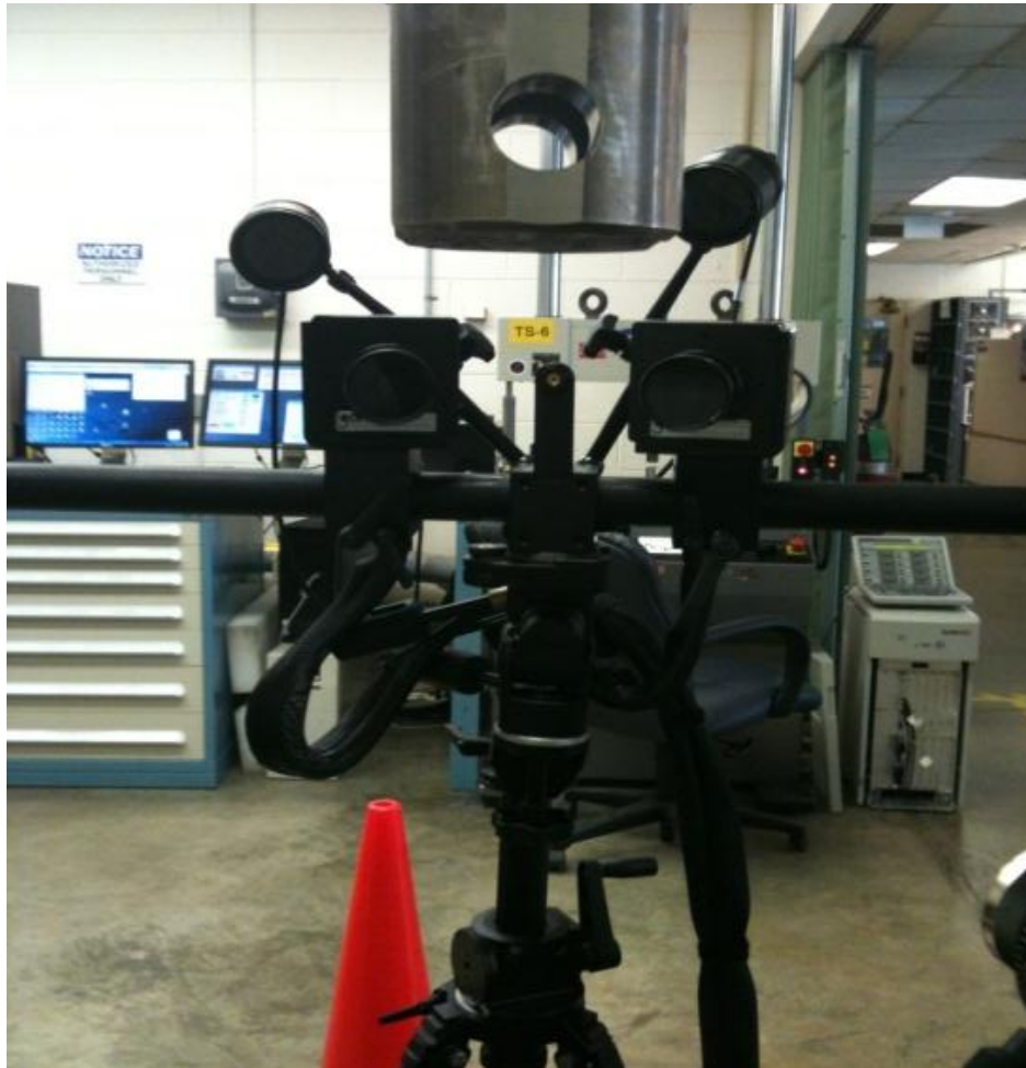
Figure B2 ARAMIS cameras used during testing.
