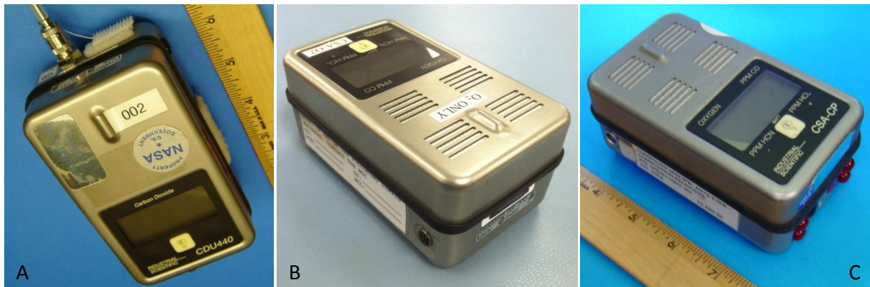
Fig 1. Three hand-held instruments in use on ISS: (A) Carbon Dioxide Monitor, (B) CSA-O2 for oxygen; and (C) CSA-CP for combustion products CO, HCN, HCl. Each is about 5x3x2 inches and weighs 1.5 lbs.
