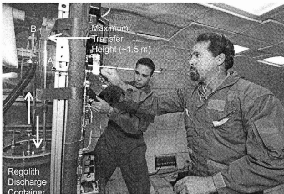
Figure 7. Photo of the RGF experiment showing Tephra that fell from cyclone A into the Regolith Discharge Container.
