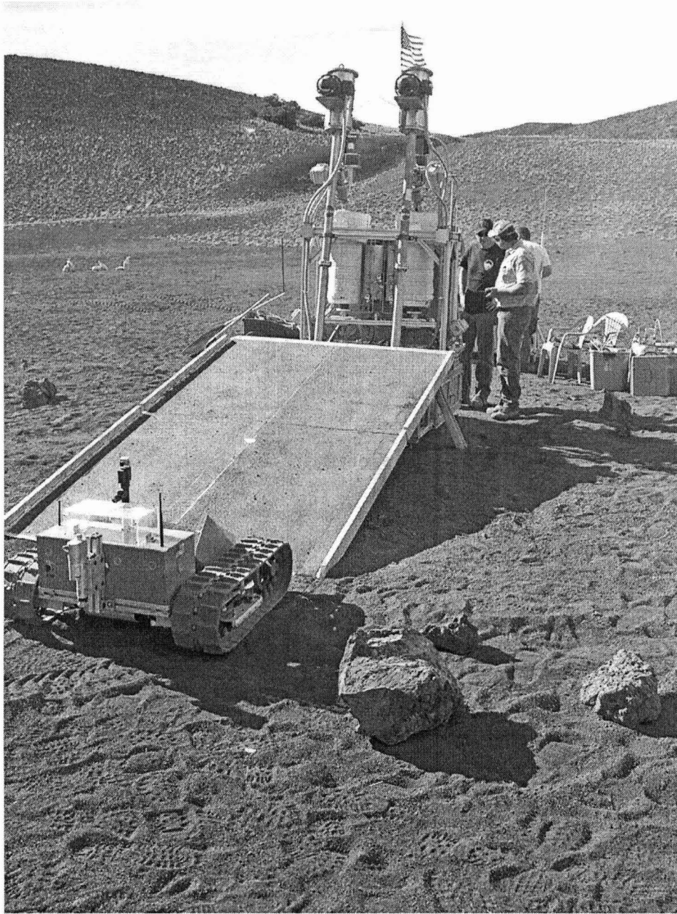
Figure 1. ROxygen I Oxygen Production Plant with an Inclined Auger RFS being Field Tested on Mauna Kea Volcano in Hawaii
