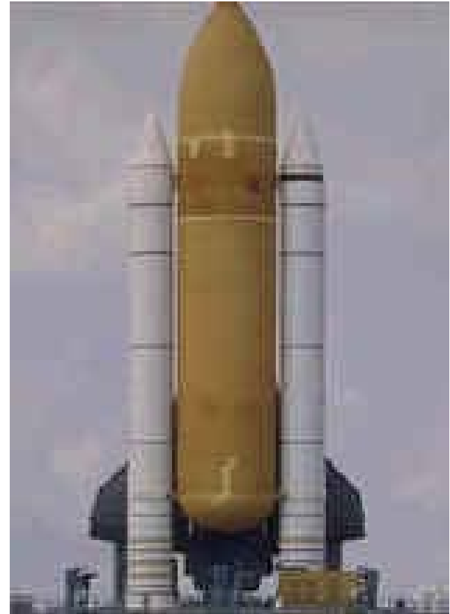
External Tank is 27.6 feet in diameter, 154 feet long.
