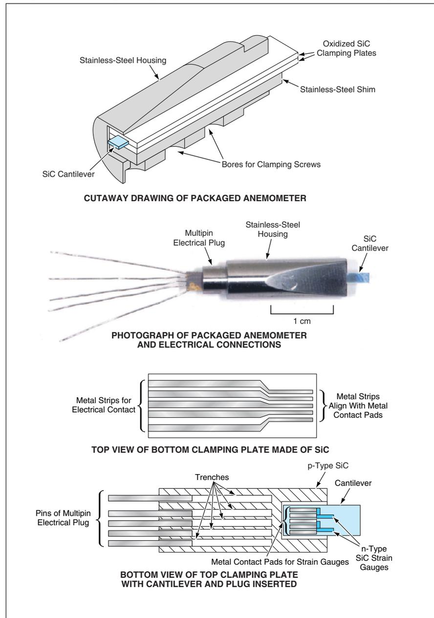
This **Cantilever-Type Anemometer** is an integral combination of functional and packaging components that, together, afford the ability to withstand high temperature, "plug-and-play" functionality, and mass-producibility.
