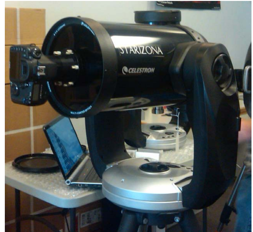
ISERV system, including Canon EOS 7D camera body; Celestron 925 CPC telescope tube and 800 CPC pointing mount; and Hyperstar 3 lens
