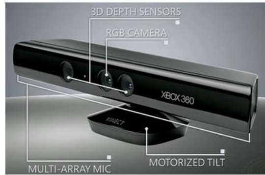
Figure 3. Locations of the various components. Depicted are the locations of the components that make up the Kinect game sensor.
