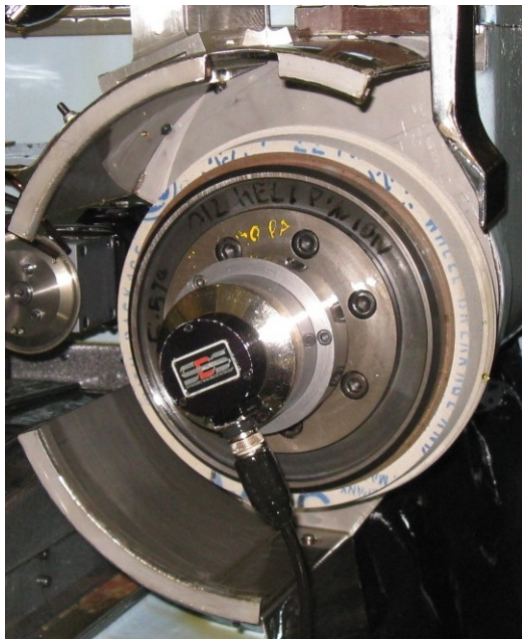
Figure 9.—Grinding wheel with dressing system.
