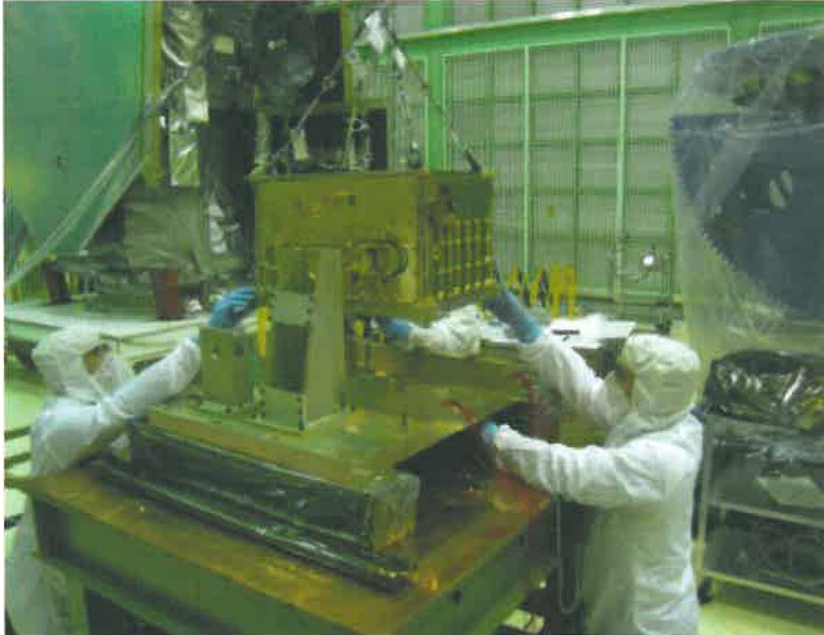
Figure 19. SAM instrument is shown being lowered on to the vibration fixture.
