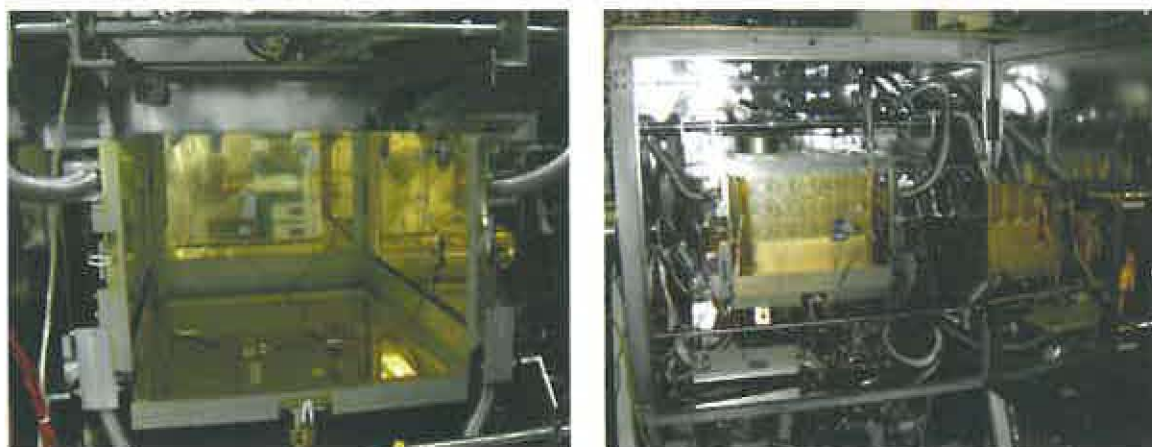
Figure 20. Picture of the SAM environmental/calibration chamber with (right) and without (left) SAM in place. The chamber itself is a cube approximately 1 meter a side.
