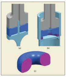
In the improved **USDC Design**, the rod was eliminated, and a solid cylinder-shaped free mass retained with a "cup" was used. On the left (a) is shown the rod configuration for the retention of the free mass, and on the right (b) the cup configuration is shown for the free mass retention. Part (c) shows a free mass with flat and curved contact areas.
