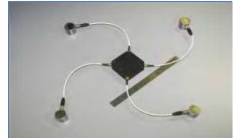
DIDS system with sensors and short cables
