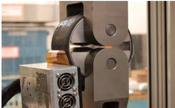
Stresses produced by tensile loading of specially design test fixture
