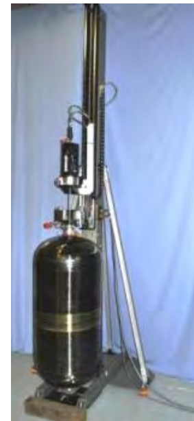
12-foot Orion Internal Profilometer developed and verified on simulator vessel
