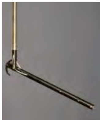
Articulated sensor developed to inspect COPV domes in NORS Internal Profilometer
