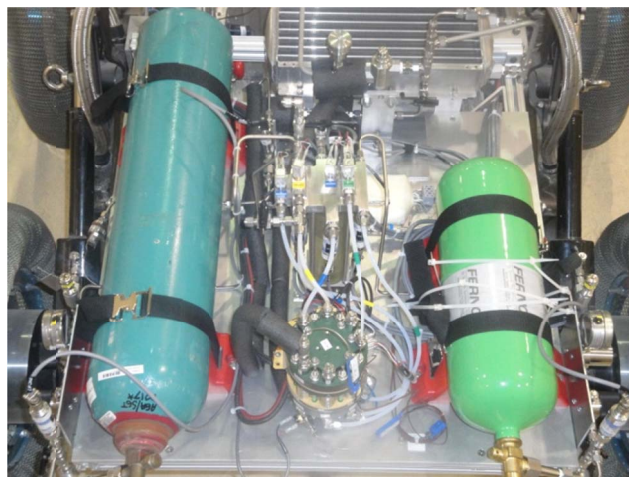
Figure 4.—Overhead view of NFT stack and reactant storage.
