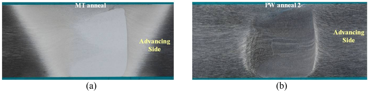
Fig. 5. Macro images of the nugget zones for MT weld after (a) MT anneal and (b) PW anneal 2.
