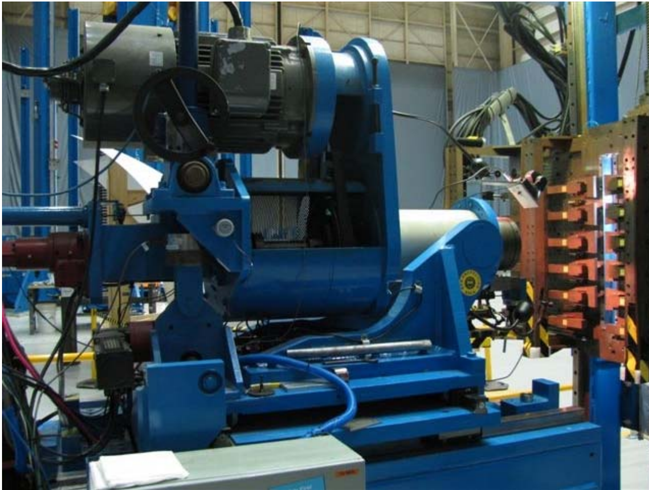
Horizontal Weld Tool used for welding development panels
