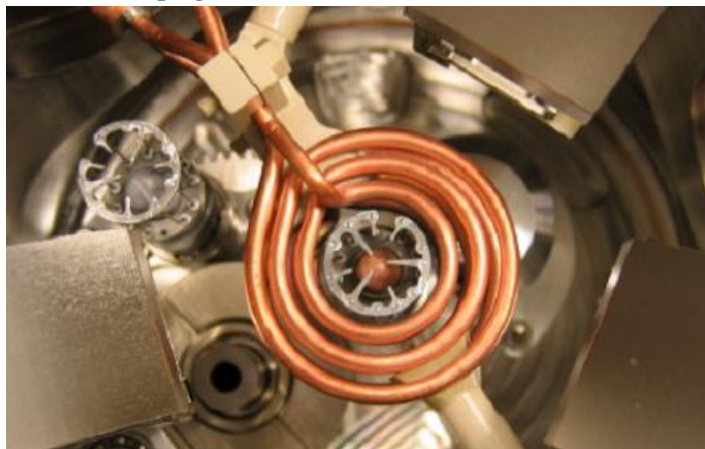
Fig. 2: EML coil and CuCo sample in a sample holder (TEXUS campaign)
