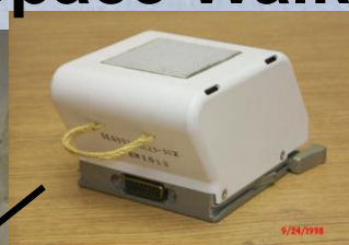
Helmet Light (EHIP) Battery Nickel Metal Hydride (NiMH)
