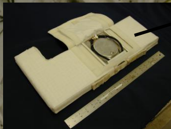
Rechargeable EVA Battery Assembly (REBA) Nickel Metal Hydride (NiMH)
